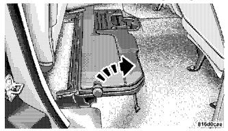
Unfolding The Load Floor 2. Grasp the knob on the load floor and lift the knob until the load floor unfolds into position.
